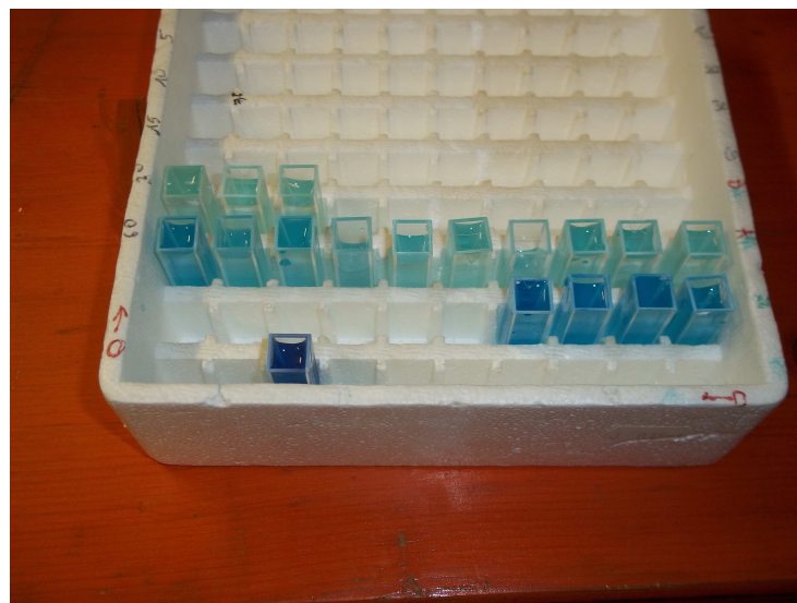
Figure 45: Photometric measured cuvettes for discoloration during the indigo method test
