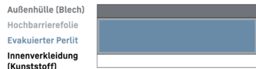
Figure 36: Structure of BluRoX vacuum insulation
